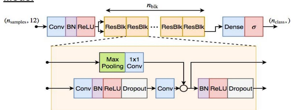
Figure: The unidimensional residual neural network (He et al., 2015) with 9 convolutional layers used for ECG classification ( $n_{\text{blk}} = 4$ ). The architecture is similar to that of Rajpurkar et al. (2017).
